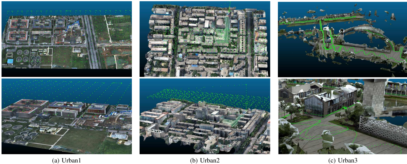
Fig. 5: The 3D texture models of the three scenes and their respective camera trajectories (green dots), in which (a) is an urban scene captured by a professional five-lens oblique photography camera, (b) is a residential scene captured by a single aerial video camera, and (c) is a business district captured by a handheld ground video camera.
