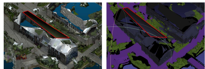
Fig. 7: A partial close-up of the texture model (left) on Urban3 and the semantic segmentation result of this part (right).
